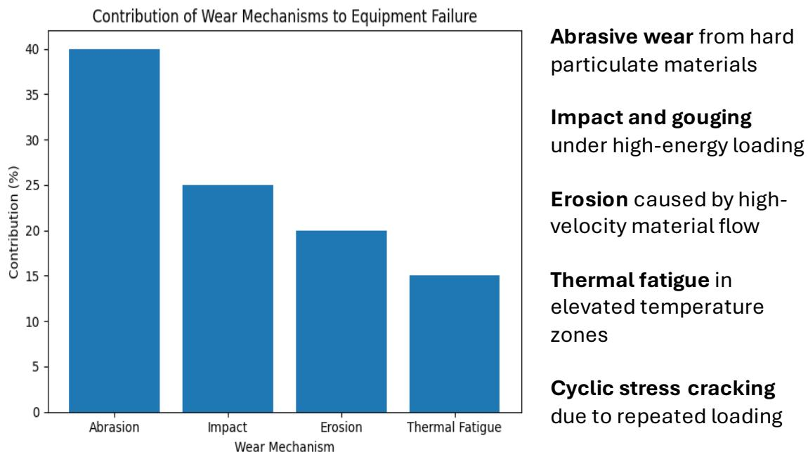
Multiple wear mechanisms act simultaneously to reduce equipment reliability in mining and bulk material handling environments (ASM International, 1992; Hutchings & Shipway, 2017).
